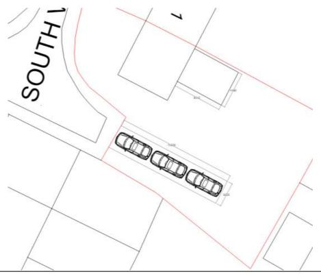
In addition, negotiations have taken place to ensure the parking area would be surfaced in permeable materials. The materials would consist of grass grid parking; a reinforced plastic permeable driveway eco paving grid which is a permeable hardstanding.
